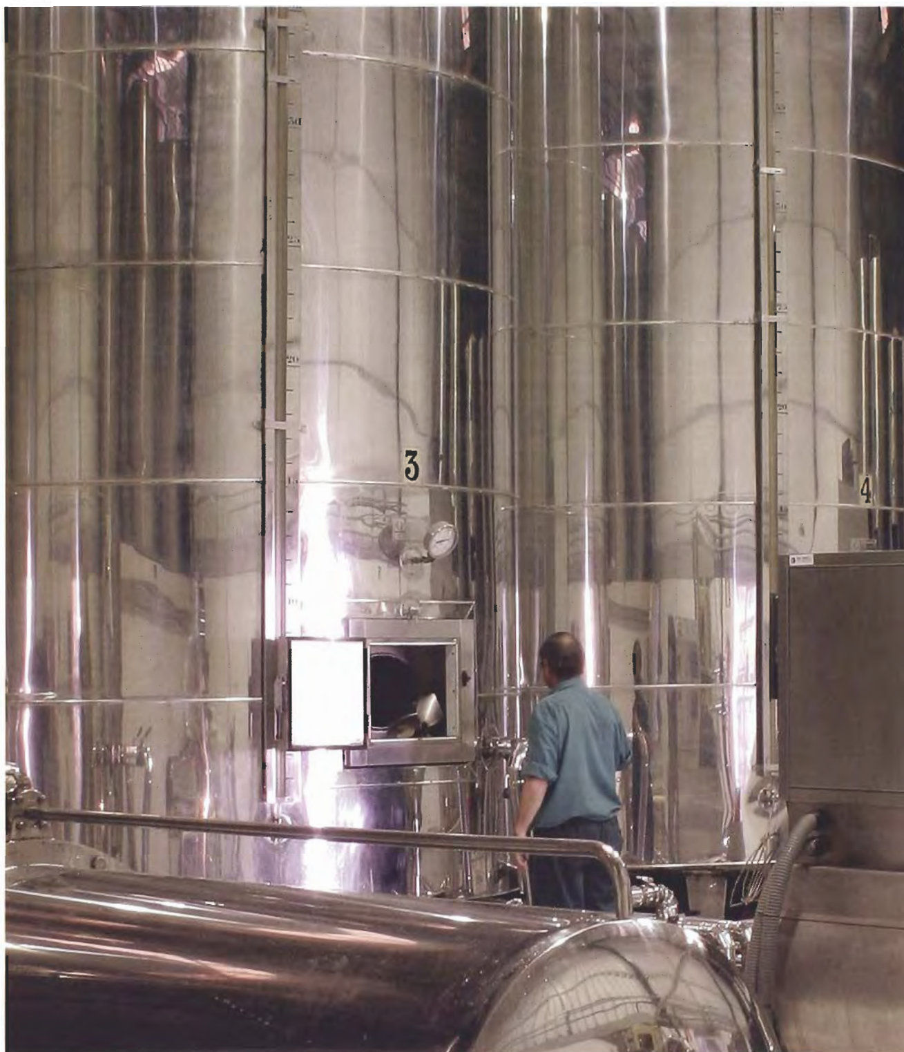
Clarified musts are transferred to fermentation tanks, where the complex process whereby sugars are turned into alcohol takes place.
